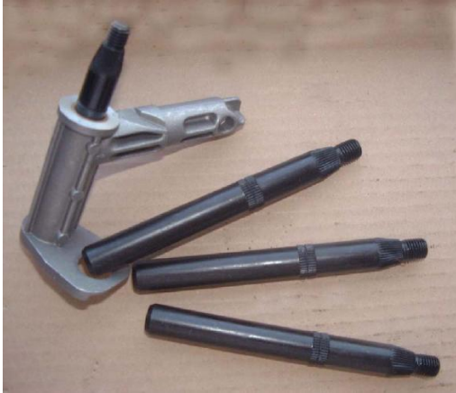
Fig. 8: CLIN treated wiper shafts
